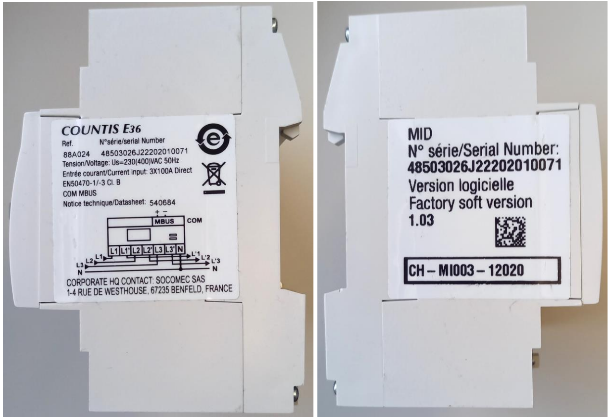
Figure 2 – Examples of type plates (on both sides)
