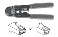
Test to ensure that all pins show continuity using a suitable appliance, RJ45 cable (8 pin test) or RJ12 (6 pin test):
