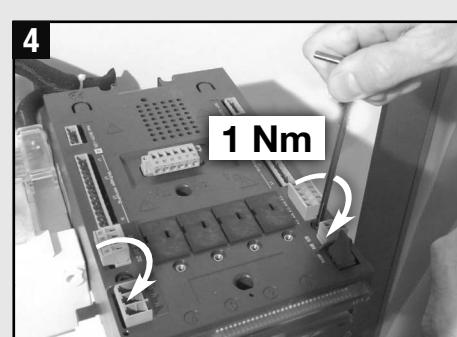
Assembling the motorisation & ATS Controller on the Power Section
