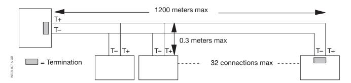
Note: T+/T- are not standard. Connection problems may be resolved by switching the + and - wires if the equipment does not operate correctly.
